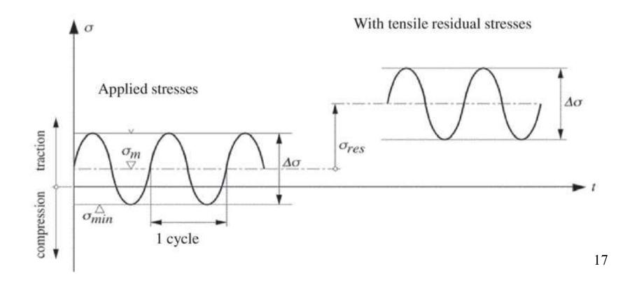
Welded details are particularly prone to fatigue because of :
