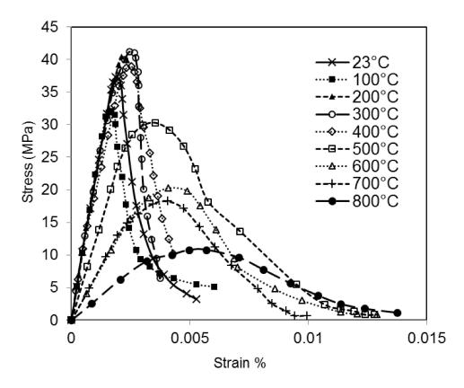
Stress-strain response (compression) of normal strength concrete at elevated temperatures
