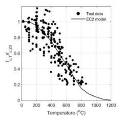
Siliceous concrete (silica, granite, sandstone)
