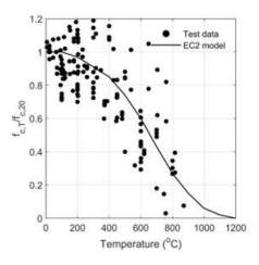
Calcareous/carbonate concrete (limestone, dolomite)
